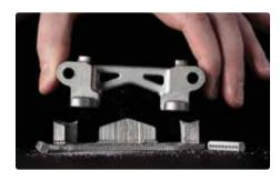
03 Ceramic release layer with anti-mold lock
